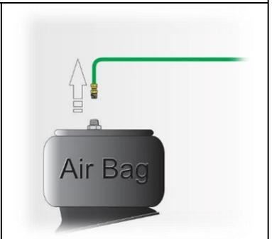
Insert the street tee fitting into the top of the air spring and then reattach the suspension air line into the Street Tee.
