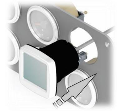
**Note:** The thickest portion of the gauge bezel indicates the bottom of the display face.
